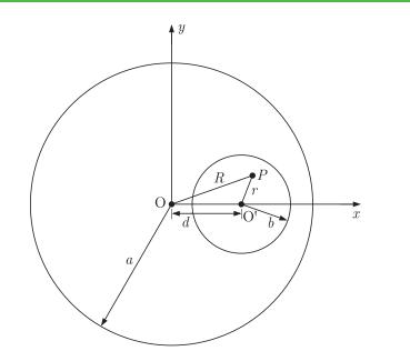
Since, the hole is drilled along the length of wire. So, it can be assumed that the drilled portion carriers current density of -J. Now, for the wire without hole, magnetic field intensity at point Pwill be given as
