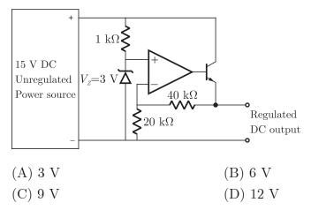
If the op-amp in the figure is ideal, the output voltage  $V_{out}$  will be equal to
