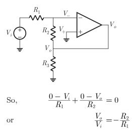
4.25 Option (B) is correct. By small signal equivalent circuit analysis
