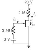
Since the FET has high input resistance, gate current can be neglect and we get  $V_{GS} = -2$  V
