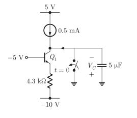
with time, the capacitor charges and voltage across collector changes from 0 towards negative.
