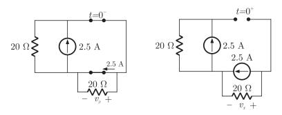
At  $t = 0^+$ ,  $i_L(0^+) = i_L(0^-) = 2.5$  A and all this current of will pass through 2  $\Omega$  resistor. Thus
