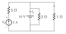
The current  $I_s$  in Amps in the voltage source, and voltage  $V_s$  in Volts across the current source respectively, are
