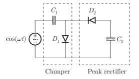
Clamper clamps the voltage to zero voltage, as shown
