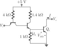
If output is at logic 0, the we have  $V_0 = 0$  which signifies BJT  $Q_3$  is in saturation and applying KVL we have
