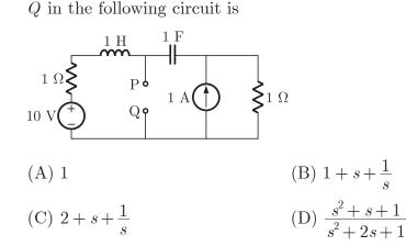
The driving point impedance of the following network is given by 2.38
