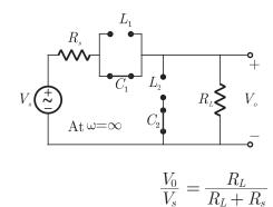
At resonant frequency  $\omega = \sqrt{\frac{1}{LC}}$  circuit acts as shown in fig and  $V_0 = 0$ .
