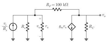
This is a shunt-shunt feedback amplifier. Given parameters,
