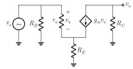
Input impedance  $R_{in} = R_B || [r_{\pi} + (\beta + 1)] R_E$  **GATE Electronics & Communication by RK Kanodia Now in 3 Volume**
