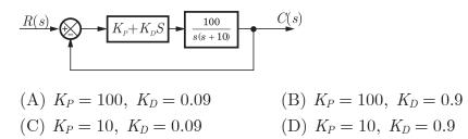
7.36 The transfer function of a plant is
