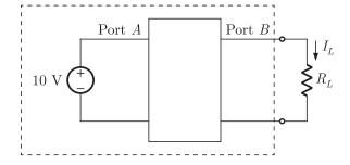
Now, we obtain Thevenin equivalent for the circuit seen at load terminal, let Thevenin voltage is  $V_{Th,10V}$  with 10 V applied at port A and Thevenin resistance is  $R_{Th}$ .
