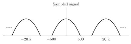
When sampled signal is passed through a LP filter of BW 1 kHz, only m(t) will remain.
