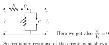
So frequency response of the circuit is as shown in fig and circuit is a Band pass filter.
