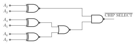
The peripheral will correspond to I/O address in the range (A) 60 H to 63 H (B) A4 to A 7H
