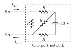
For a one port network current entering one terminal, equals the current leaving the second terminal. Thus the outgoing current from A to B will be equal to the incoming current from D to C as shown
