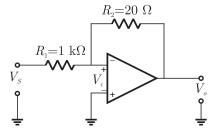
Let V be the voltage of inverting terminal, since non inverting terminal a at ground, the output voltage is
