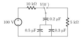
$V(0^{-}) = 100 \text{ V}$ Thus  $V(0^{+}) = 100 \text{ V}$ At  $t = 0^{+}$ , the circuit is as shown below
